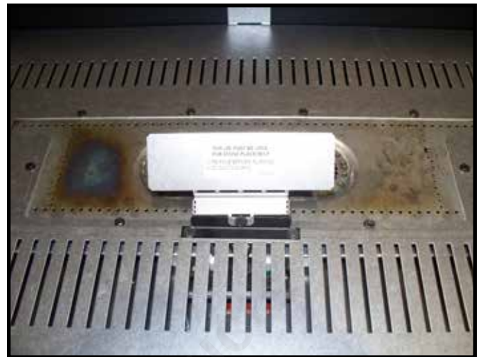
Figure 14.5 Rock Fixture Assembly Installed
