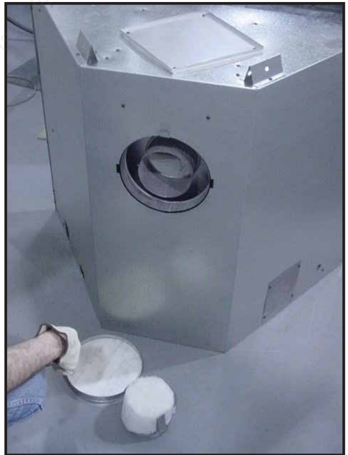
Figure 9.11 Discard the vent cap, remove and discard the insulation basket.
