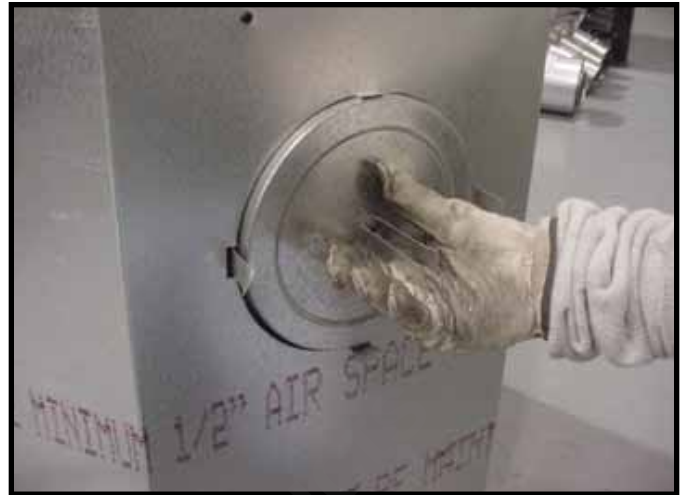
Figure 9.10 Fold the center parts of the retaining band out and use to remove the seal cap.
