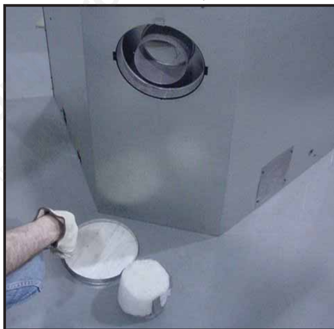
Figure 9.11 Discard the vent cap, remove and discard the insulation basket.
