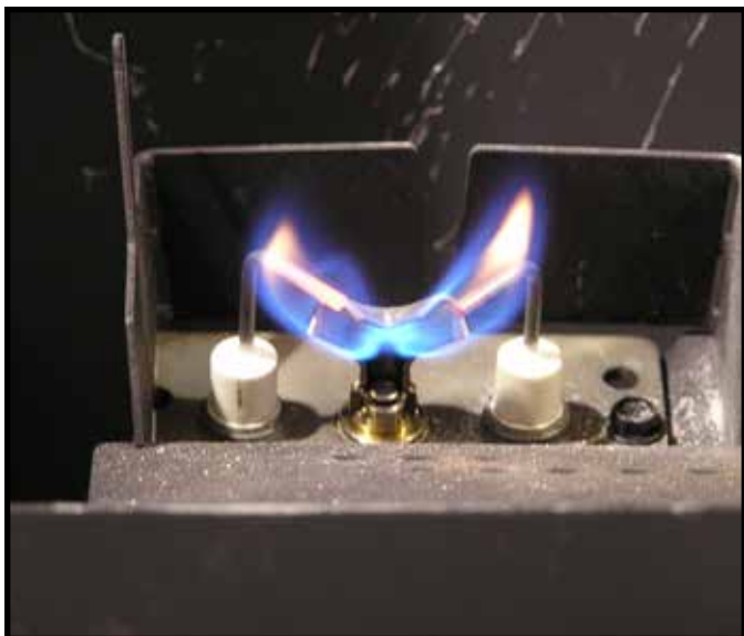
Figure 3.1 IPI Pilot Flame Patterns
