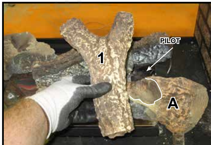
Figure 3. Placement of Log #1
