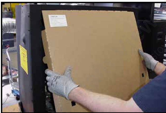
Figure 11.5 Installation of Splatter Guard
