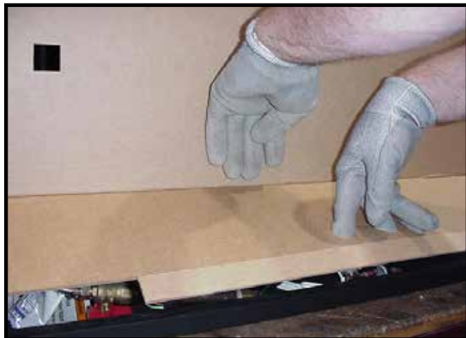
Figure 11.9 Opening Lower Access Panel
