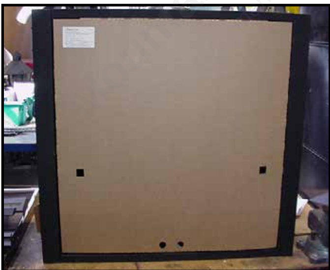
Figure 11.12 Splatter Guard with Lower Access Panel Closed
