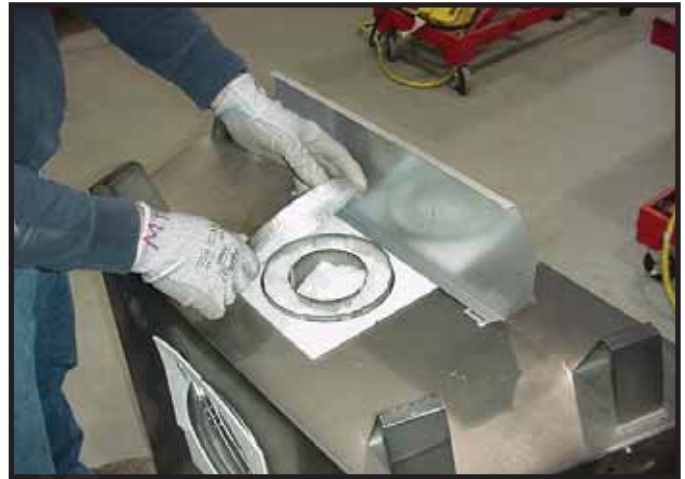
Figure 9.4 Remove the seal cap.
