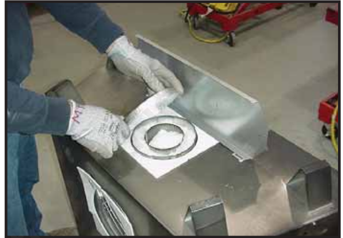
Figure 6.4 Remove the seal cap.
