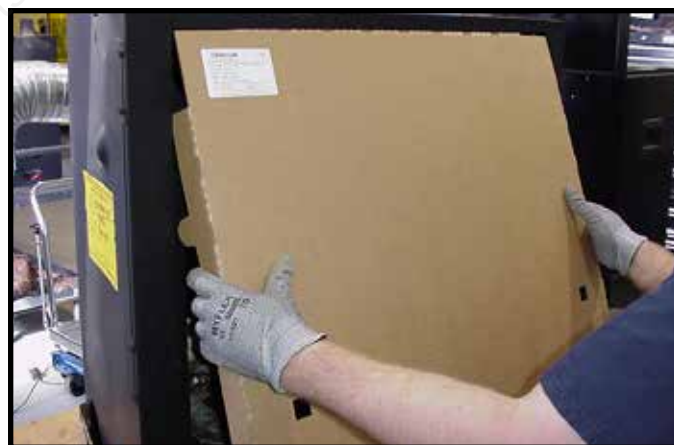
Figure 13.4 Installation of Splatter Guard
