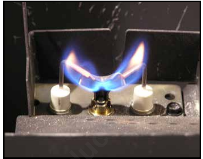
Figure 3.2 IPI Pilot Flame Patterns
