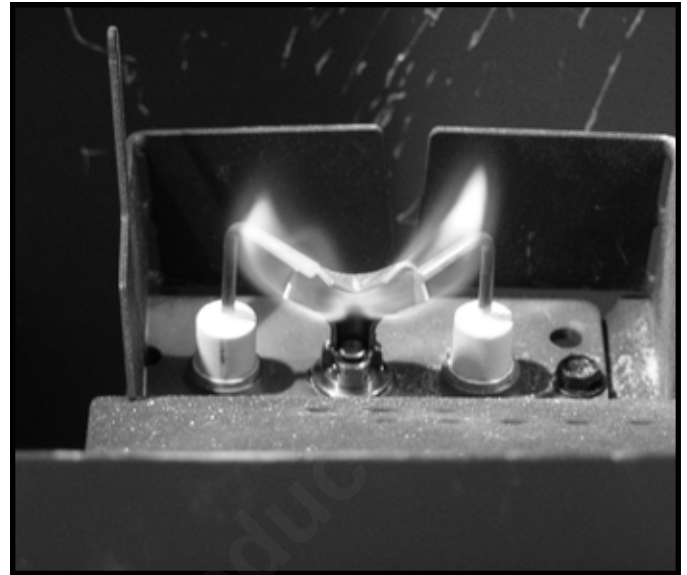
Figure 4.2 IPI Pilot Flame Patterns - Generic Photo
