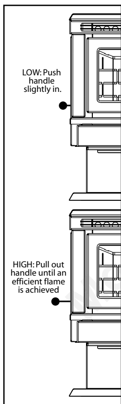
Figure 1: Slider / damper positions.
