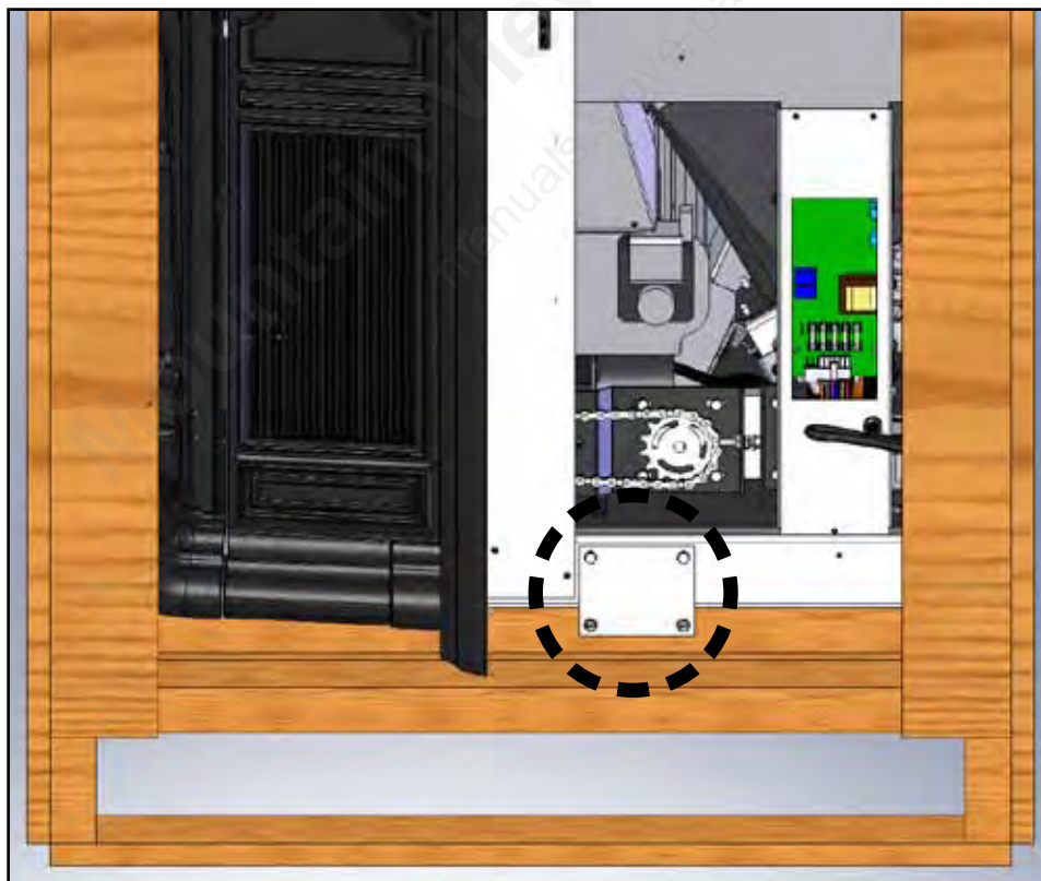
Figure 3: Mounting Plates securing stove to pallet
