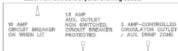
Label from unit control panel showing outlets
