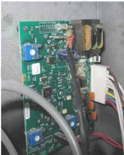
The optional Room Sensor cable attaches to two bare terminals on the rear of the circuit board. These connections are not polarity specific.
