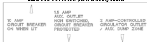
Label from unit control panel showing outlets
