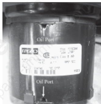
Figure 24. Oil ports on a circulation fan
