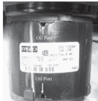
Figure 24. Oil ports on a circulation fan
