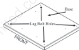
Figure 16C KSH Anchor Holes
