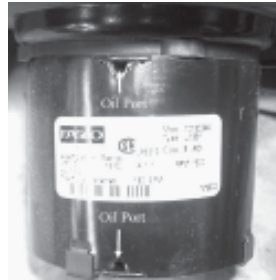
Figure 22. Oil ports on a circulation fan
