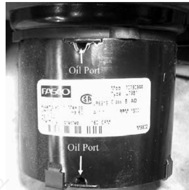
Figure 19. Oil ports on a circulation fan
