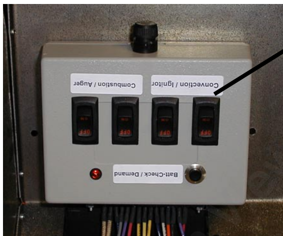
TEST BOX (AS IT IS INSTALLED IN THE STOVE)
