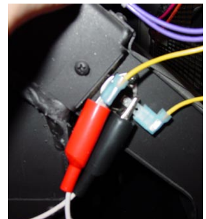
#2 SNAP DISC WITH A JUMPER WIRE ATTACHED.
