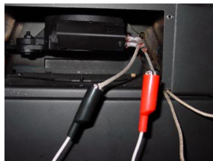
CLIPS HOOKED UP TO THE IGNITER
