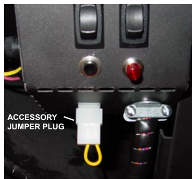
ACCESSORY JUMPER PLUG ON THE JUNCTION BOX.
