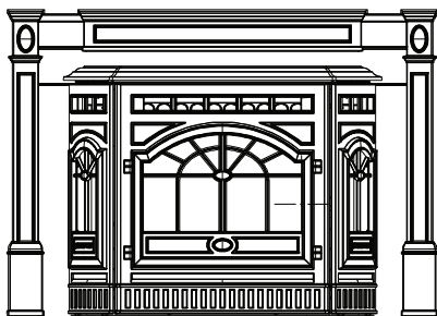
Figure 21.2 - Completed View of Panel Set & Cast Trim Set
