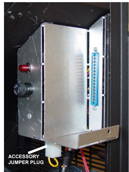
ACCESSORY JUMPER PLUG ON THE JUNCTION BOX.
