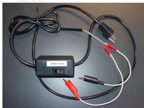
TEST CORD w/ CLIPS ATTACHED
