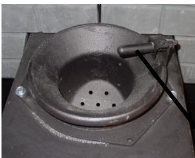
THERMOCOUPLE TIP WITH PROTECTIVE COVER
