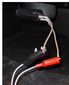
CLIPS HOOKED UP TO THE IGNITER
