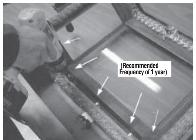
Figure 40 - Remove Window Wash Bracket (5 screws)
