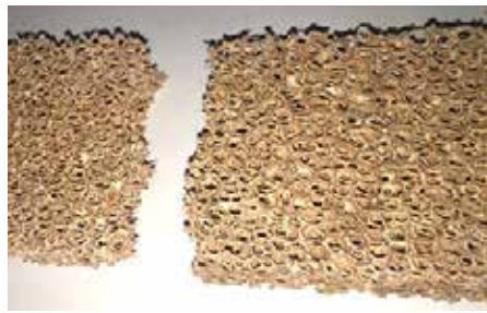
Combustor Problem - Broken Combustor
