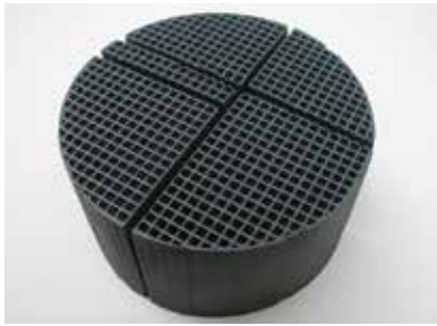
Photo #4 Mechanical Cracks
