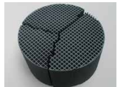
Photo #3 Thermal Cracks
