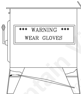
3- Install the heat shield between the front legs, just above the leg supports.
