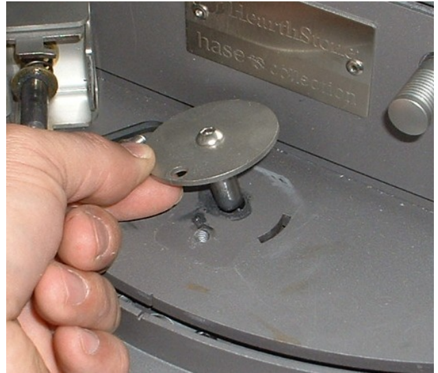
Figure 6: Insert Rotation Lock
