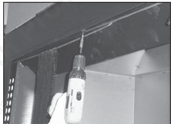
Figure 4.8 Removing the Screen Rods
