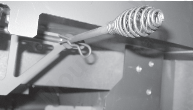
Figure 4.25 Reinstalling Hairpin Clip and Washer
