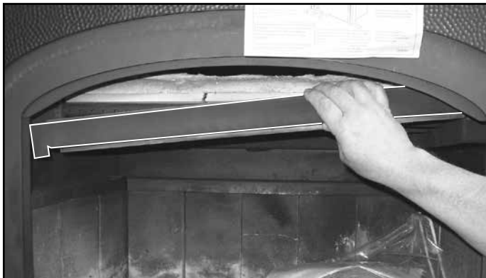
Figure 4.5 Removing Baffle Protection Channel
