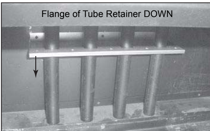
Figure 10 Place and Fasten Tube Retainer
