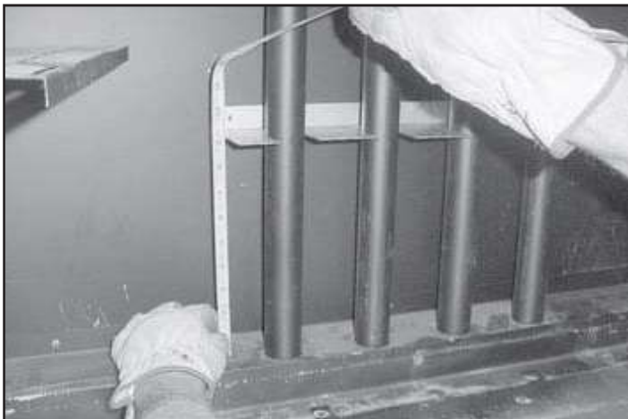
Figure 9 Fasten Center Tube Support
