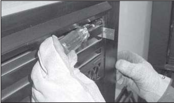
Figure 3 SC60 Remove Upper Grille
