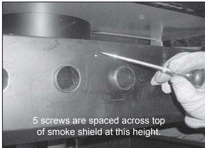
Figure 17 EM-42 only - Check for Screws in Smoke Shield
