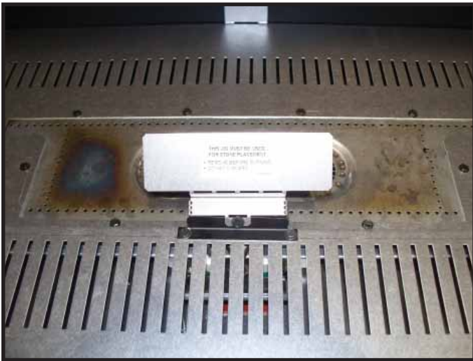
Figure 11.6 Rock Fixture Assembly Installed
