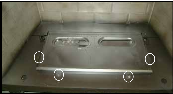
Figure 3.9 Remove Burner Skirt
