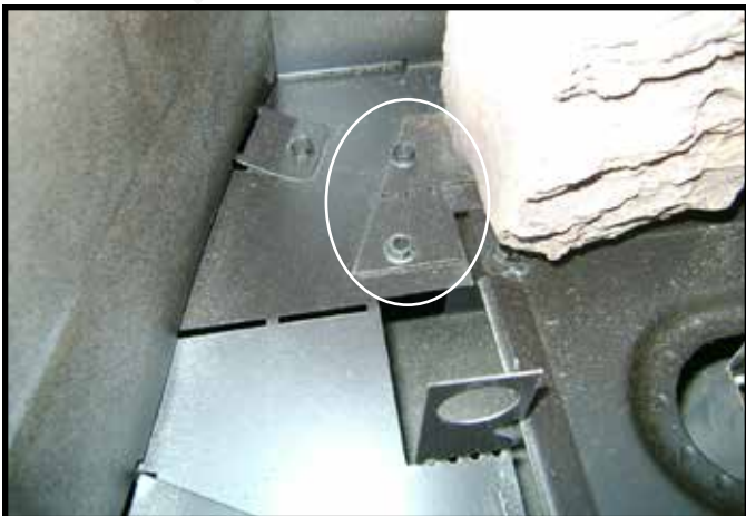
Figure 3.4 Remove Screws from Log Tabs
