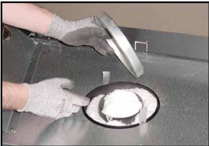
Figure 9.3 Remove the seal cap.
