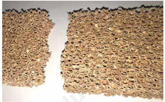
Combustor Problem - Broken Combustor
