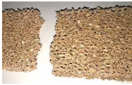
Combustor Problem - Broken Combustor
