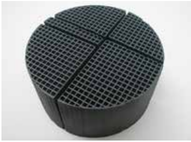
Photo #4 Mechanical Cracks
