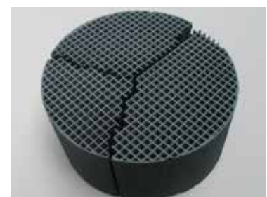
Photo #3 Thermal Cracks
