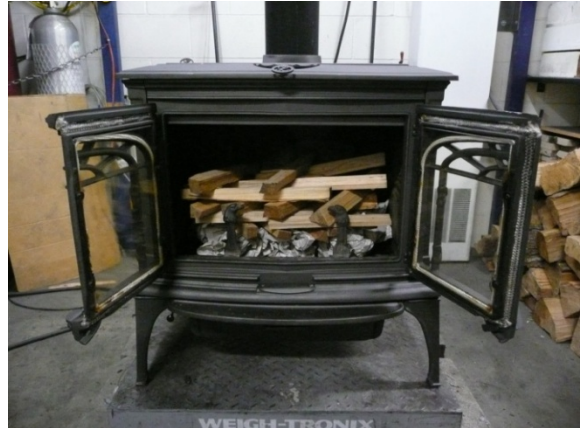
Stack 10 to 20 pieces of kindling on top of the newspaper in a criss cross pattern to allow plenty of air flow.
