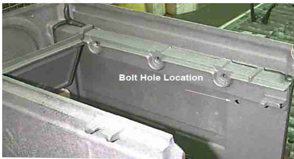
Remove right secondary air channel
