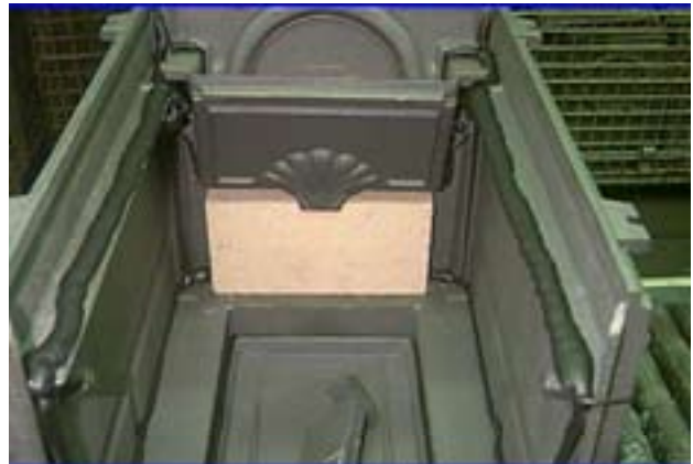
Sides installed with rear brick
