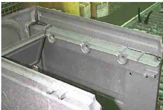
Right secondary air channel ready for bolt
