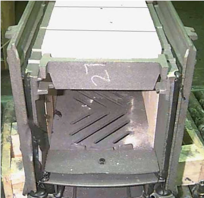
Assembly with bricks, air manifold, grate and deflector installed
