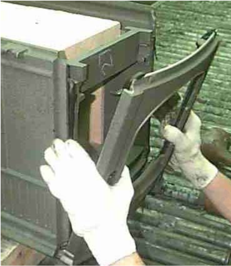
Assemble stove front panel
