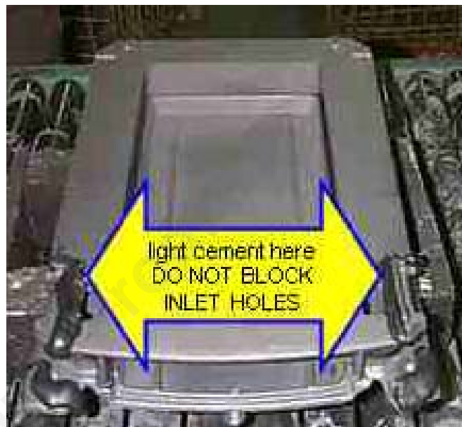
Inner bottom installed
