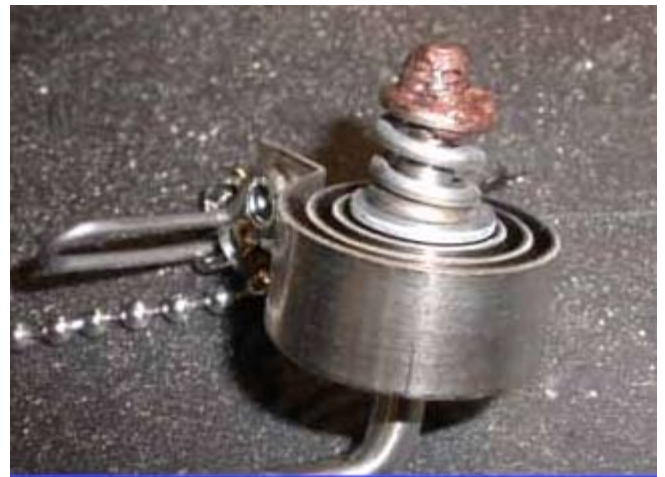
Install washer, spring and anti-seize
