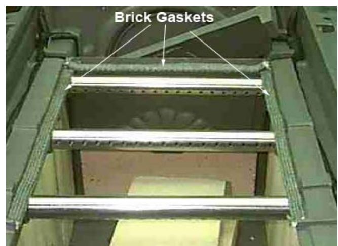
Remove brick gaskets and secondary air tubes
