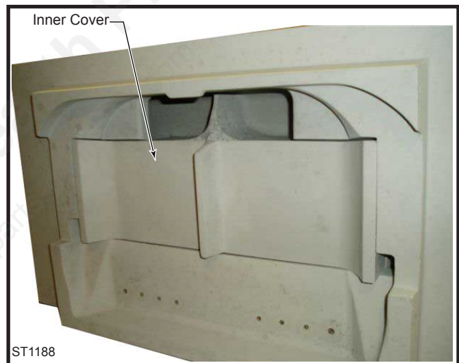
Fig. 29 Remove inner cover.
