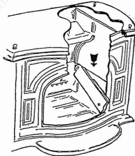
FIG. 2 SLIDE UPPER BAFFLE DOWNWARD
