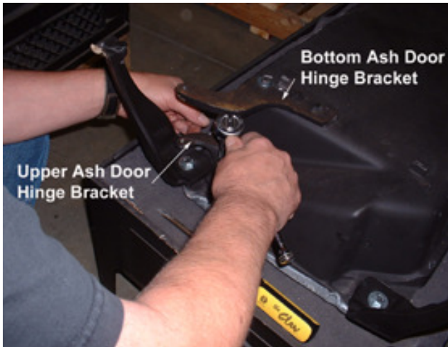
Fig.5 Attach Ash Door Hinge Brackets
