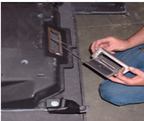
Fig. 8 Primary Air Valve Attachment
