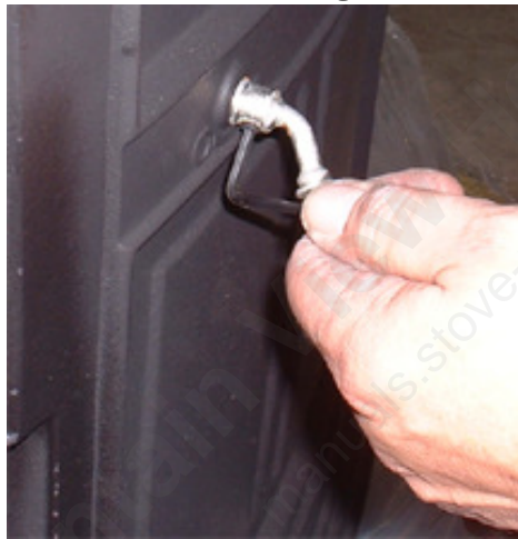
Fig.1 Remove Primary Air Handle
