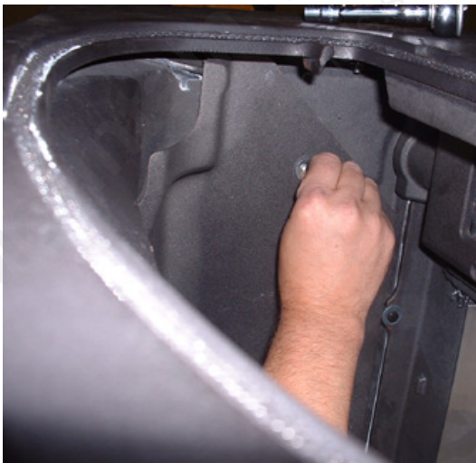
Fig. 25 Install Left Air Plate
