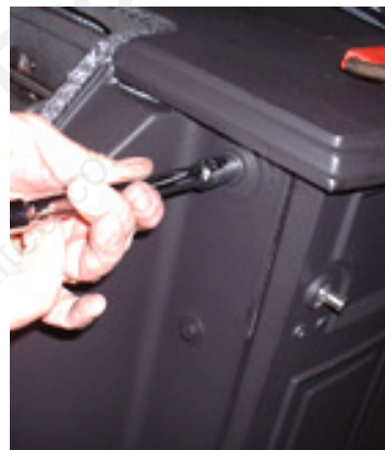
Fig. 21 Install Upper Fireback Bolts
