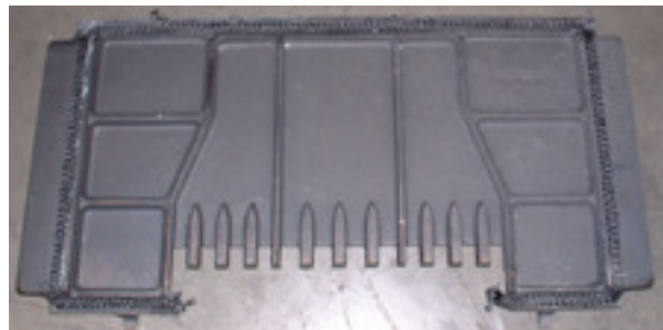
Fig. G-11 Lower Fireback Rear View 5/16" x 55" Fiberglass lower fireback to upper fireback and rear
