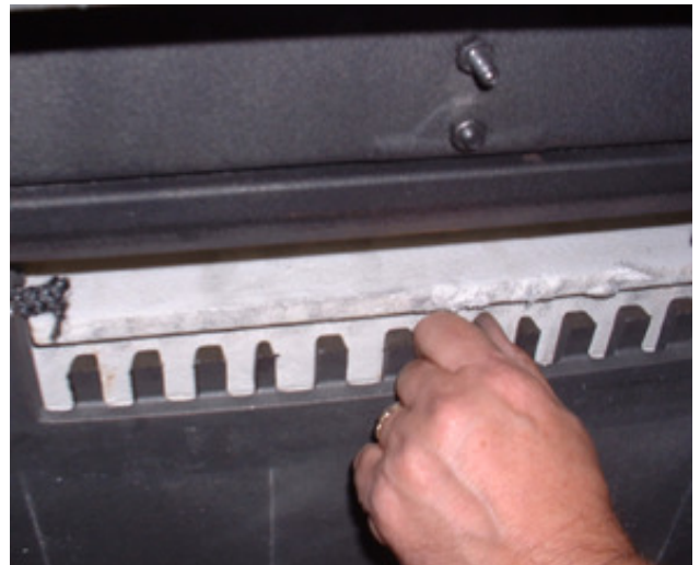
Fig. 26 Install Upper Fireback
