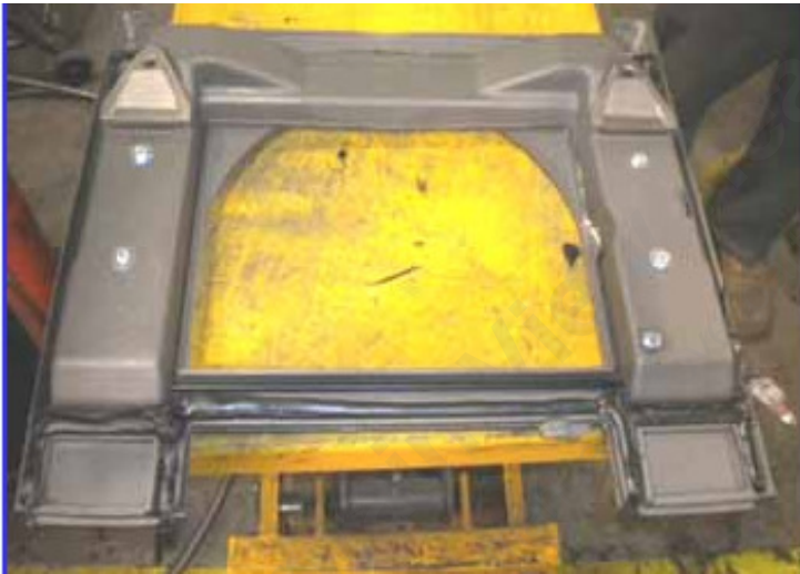
Install Furnace Cement Bottom View
