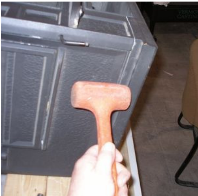
Fig. 3 Strike the outer bottom to release it and pull it off
