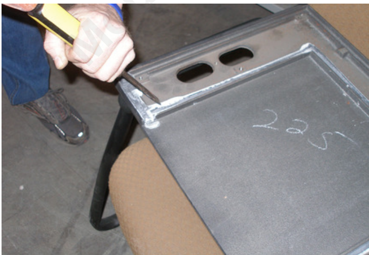
Fig. 5 Clean the grooves of the outer bottom
