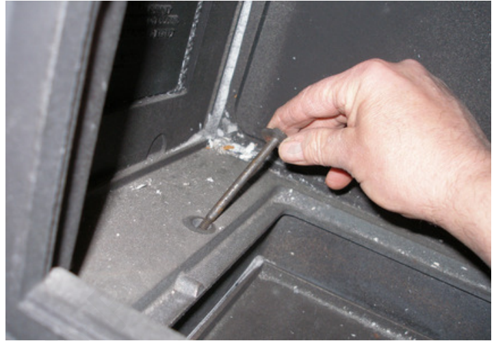
Fig. 8 Replace the two bolts and washers holding the outer bottom to the inner bottom
