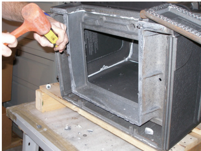
Fig. 6 Clean the ends of the inner bottom
