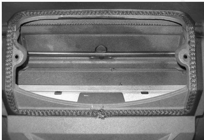
Insulator Board - 30005269 bolted to back
