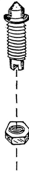
Fig R-10 DETAIL OF THE LOWER LOADING DOOR HINGE PIN AND LOCK NUT
