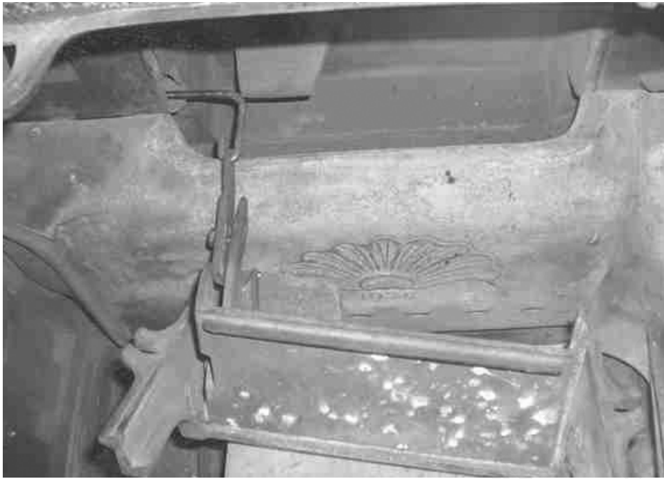
Fig. 14 Upper Fireback damper handle position
