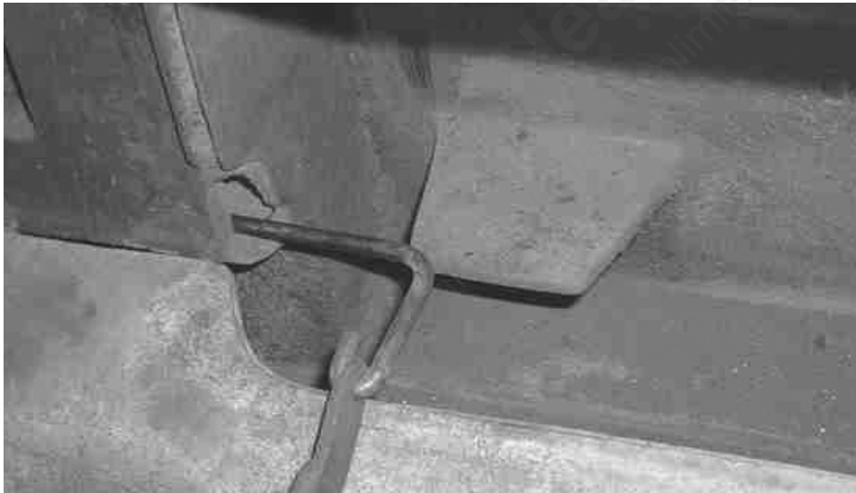
Fig. 15 Damper Link and Damper Handle close up
