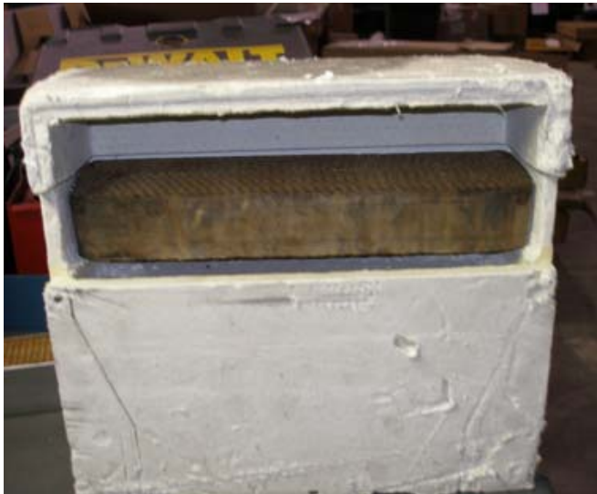
Front View of Refractory Assembly # 1602510 with included access panel (1602511) removed showing the catalyst installed
